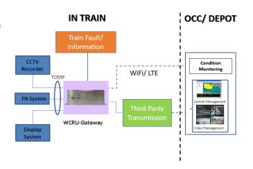
The WCRU-Gateway, operating as communication gateway of the vehicle, enables Access Control Security with User ID and Password with audit trail to remote stations for any kinds of applications in the train which can be connected via its customizable communication suite. Multiple devices can directly be attached to the WCRU-Gateway by using the integrated 5 Ethernet.
