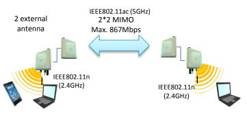
**AP-8010NAC-2E2S** is able to support 2 radio streams up to 867Mbps wireless data rate
